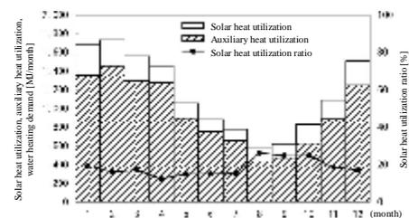
Figure 2 Quantity and ratio of solar heat utilization (calculated values)
