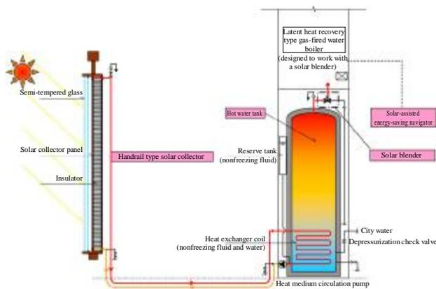
Figure 1 Outline of the next-generation solar-assisted water heating system
