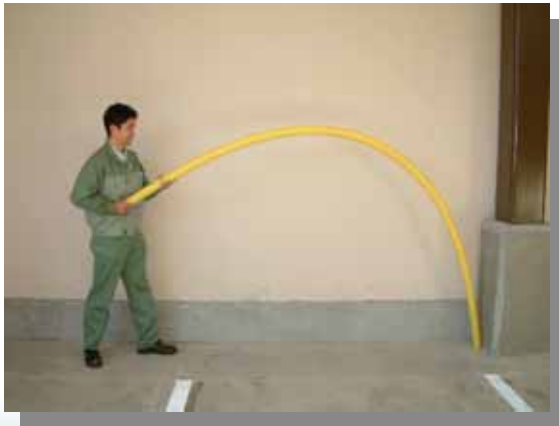
A polyethylene pipe that can follow even a large ground displacement
