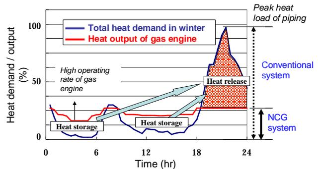
Fig.3 The effect of time leveling of heat supply.
