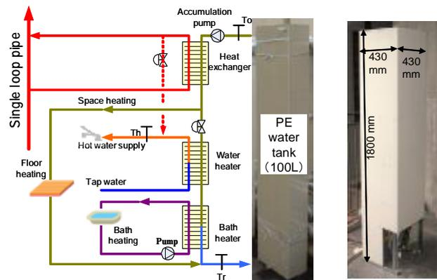
Fig.4 Flow and external appearance of the heat storage unit.
