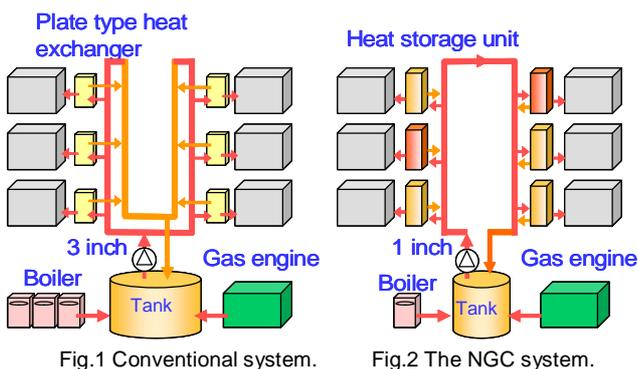
On the other hand, the NCG system installs a new heat storage unit equipped with a hot water supply and a space heating function in every household, and these units are interconnected by a small one-inch single-loop pipe. Hot water is circulated full time at the flow rate of an inverter pump controlled by heat load of the single-loop pipe as shown in Fig.2.
